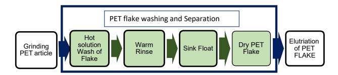
A material balance evaluation must be conducted by an to verify the efficiency and loses of the washing and separation process by streams.
