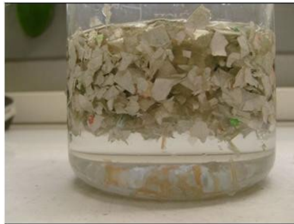
Photo 3: Sink float separation of regrind labels sample
