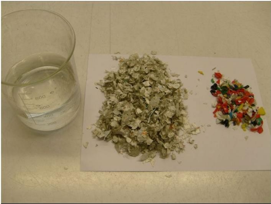
Photo 1: From left to right, beaker with 300 ml water at pH 7,5; label sample; regrind caps sample
