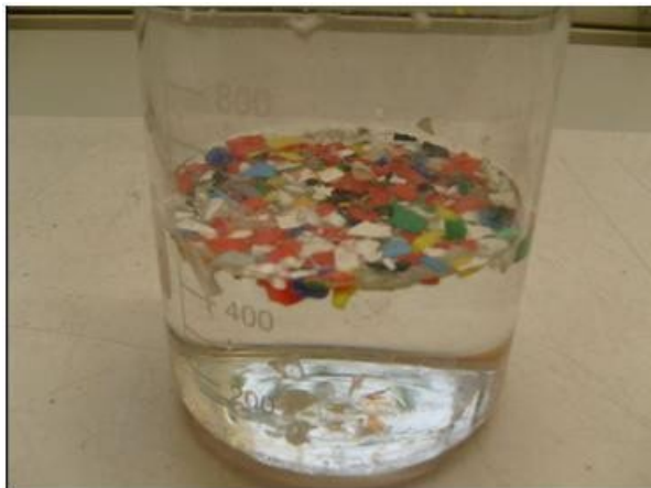
Photo 2: Sink float separation of regrind caps sample
