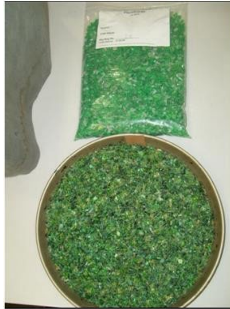
Photo 2: Flakes before and after oventest
