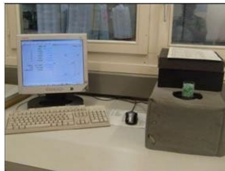
Photo 8: Minolta spectrophotometer (optional)
