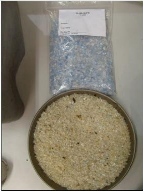
Photo 1: Flakes before and after oventest
