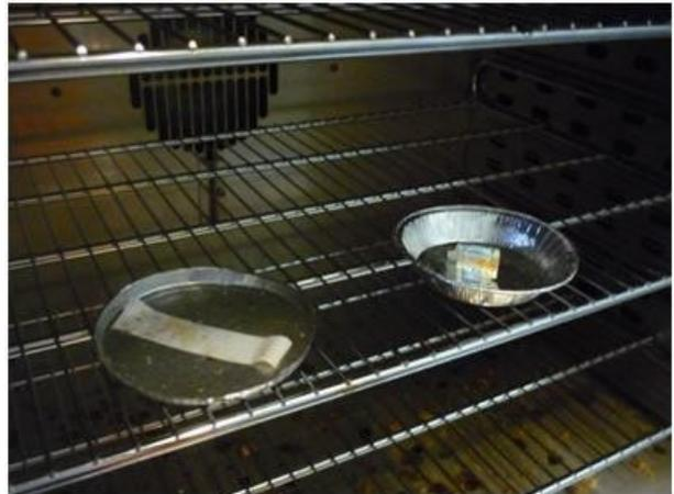
Photo 4: Dry sample for 2 hours at 85°C (W1)
